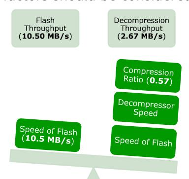
If Flash throughput is greater than decompression throughput then an uncompressed image is quicker
